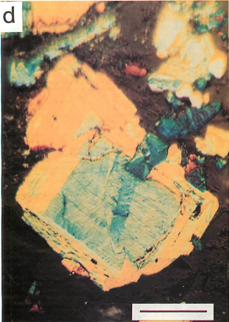
FIG. 3d. Optical micrograph of stained arsenopyrite grain from Fairview mine showing color contrast. Scale bar is 0.1 mm.
